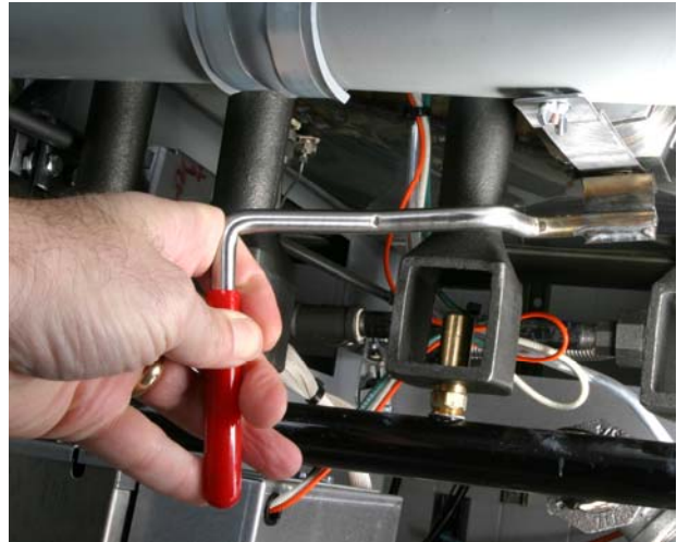
Moving the red drain valve handle to open the drain valve, allowing hot oil to drain into the filter pan.
